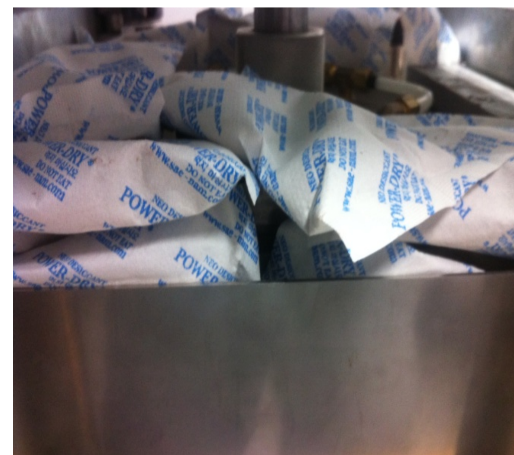
Moisture sensor in shear box Shear box with Crushed mudstone covering by Silica gel
