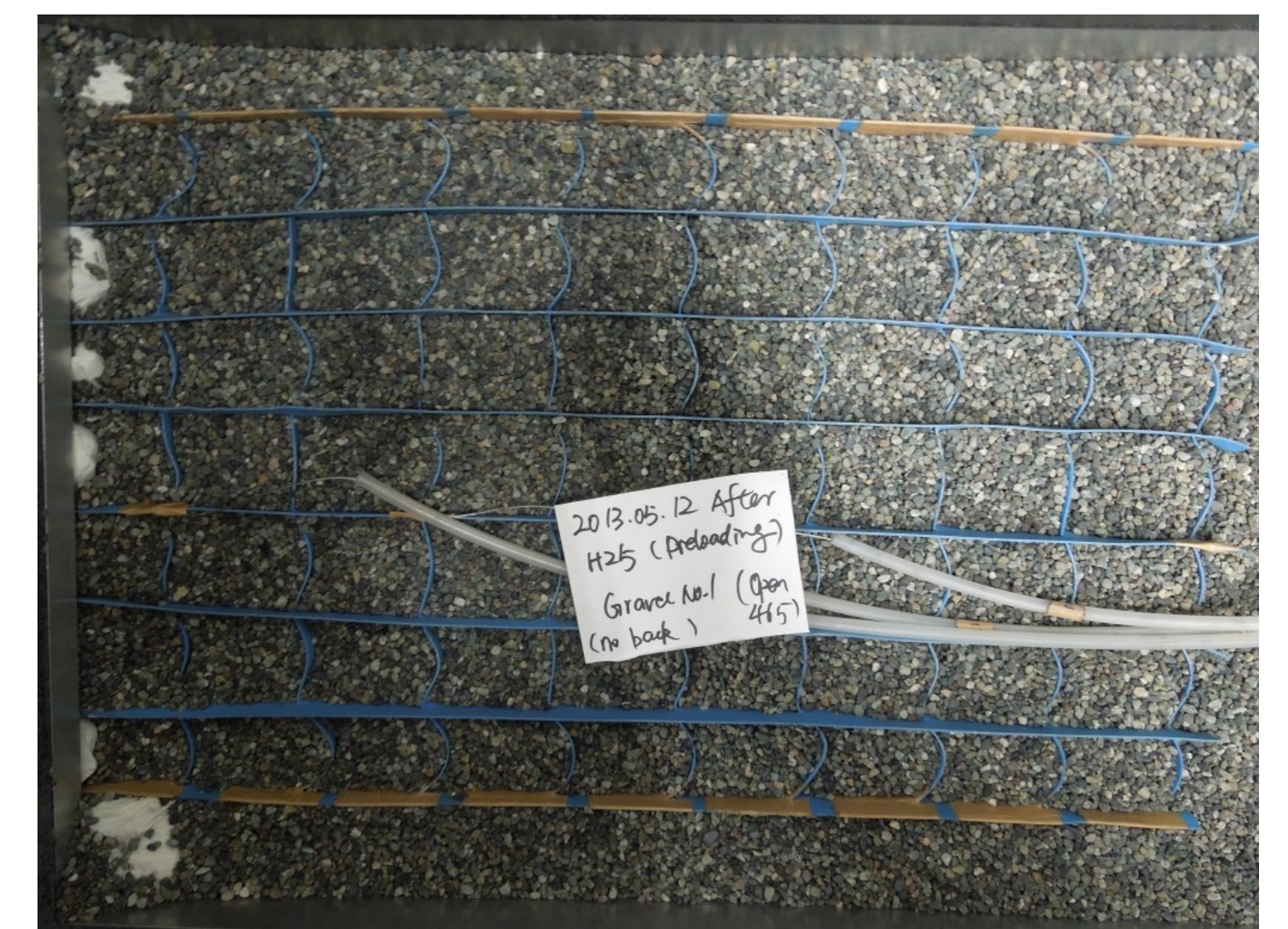
Comparison of arrangements of geocell members before and after pullout test
