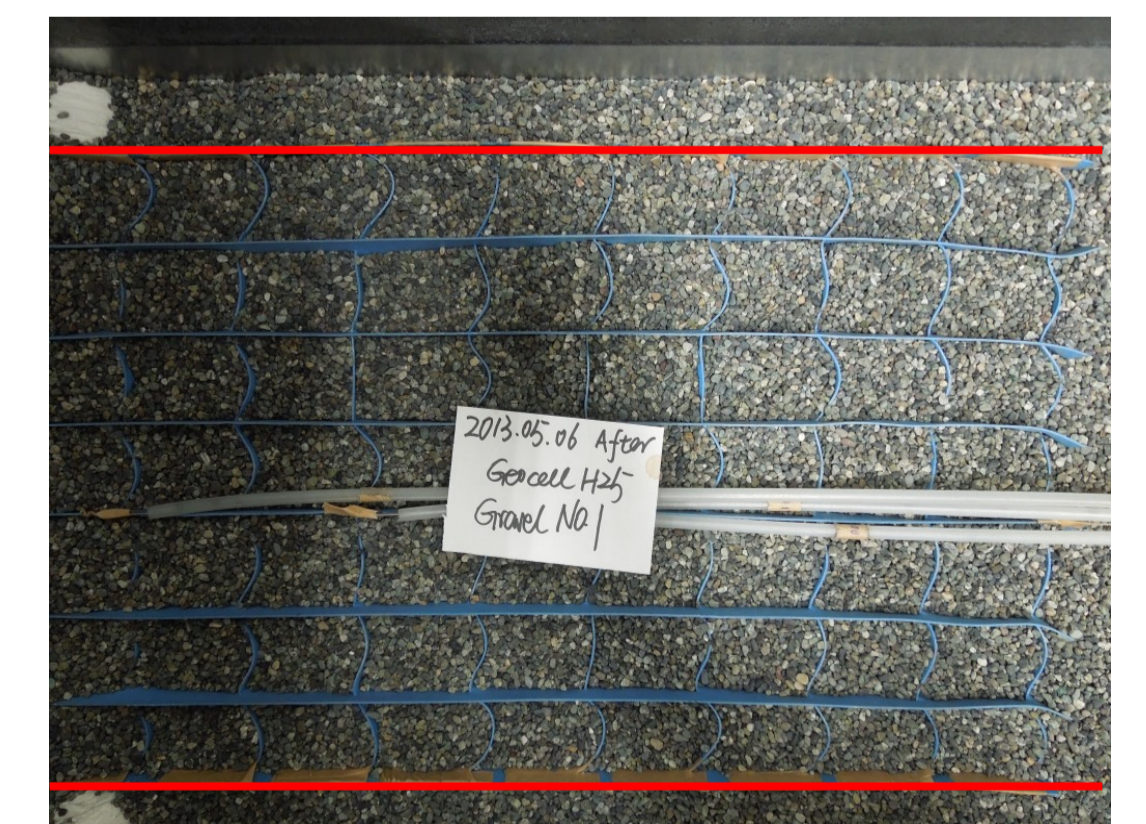
After tests, the deformation state of diamond-shaped geocell and square-shaped geocell
