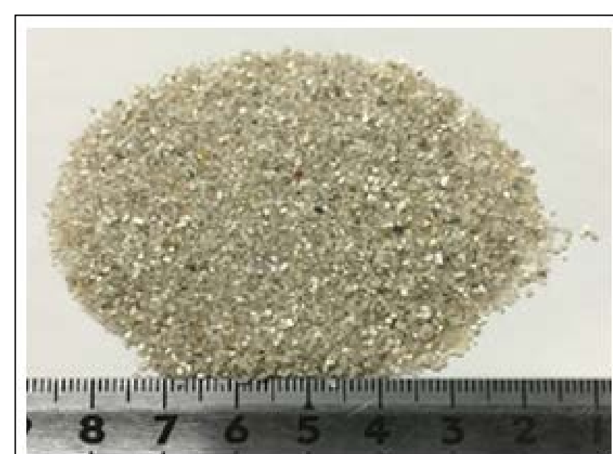
Fig.2. Sand No.5 ( D_{50}=0.64\text{mm} )
