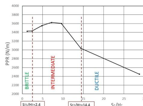
Fig. 7 - Threshold limits of the 3 failure modes
