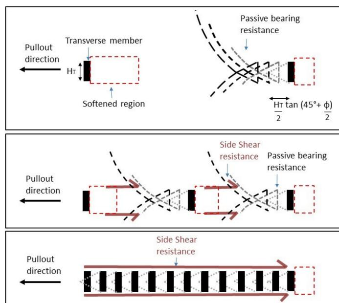
Fig. 4 - Conceptual mechanism (3 failure modes depending on  $S_T$ )
