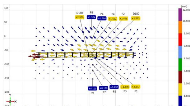
Fig. 6(c) - Deformation of S30 at peak (at 180 S,  $D_{180} = 2.5\text{mm}$ )
