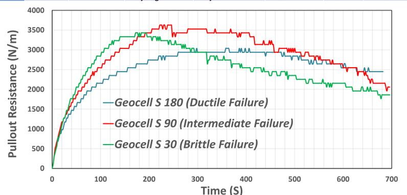
Fig. 5 - Typical failure patterns
