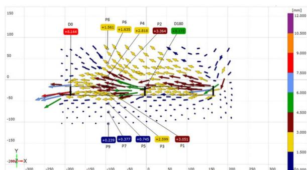
Fig. 6(a) - Deformation of S180 at peak (at 360 S,  $D_{180} = 5\text{mm}$ )
