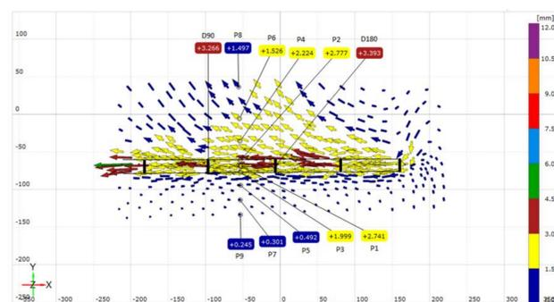
Fig. 6(b) - Deformation of S90 at peak (at 247 S,  $D_{180} = 3.5\text{mm}$ )
