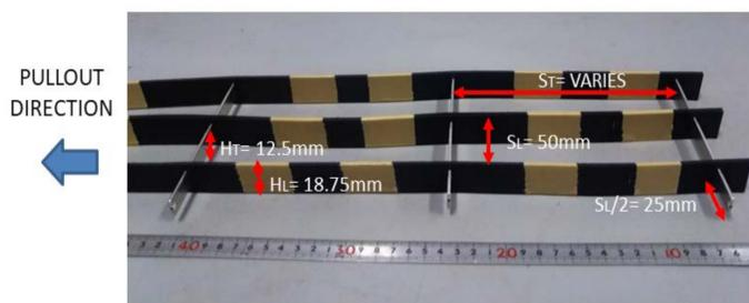
Fig. 2 - Split-type geocell reinforcement
