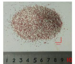
Fig. 3 - Backfill material (Colored sand No5)
