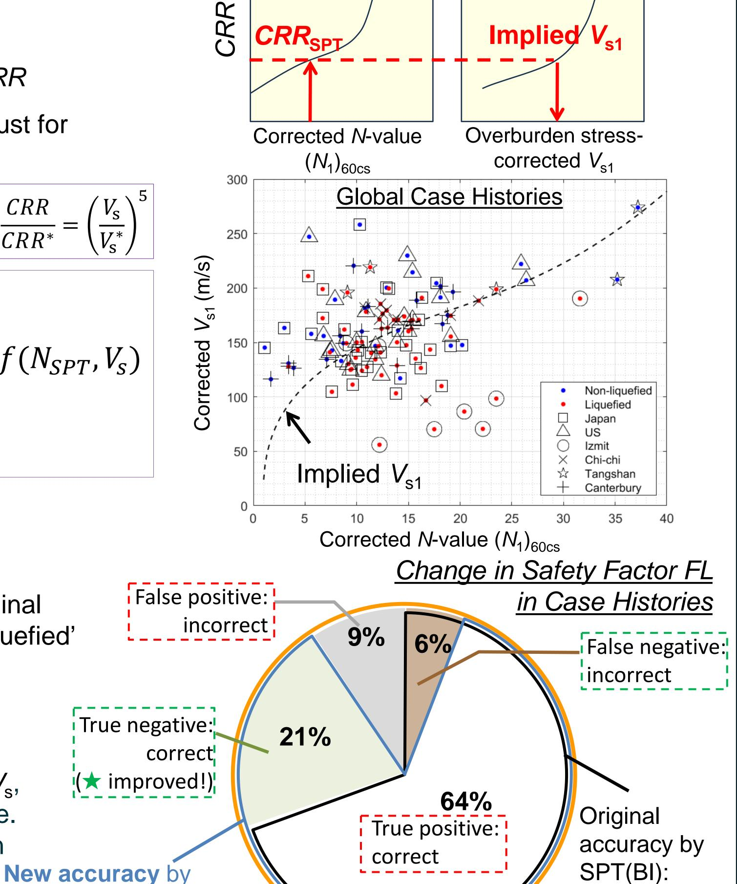
$$CRR_{SPT,V_{S}} = f(\text{density, soil fabric}) \cong f(N_{SPT}, V_{S})$$
